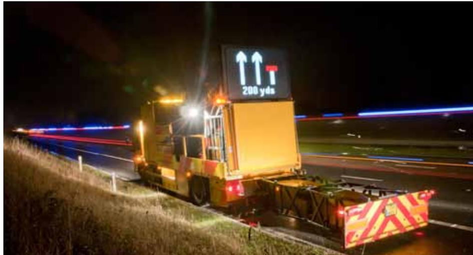
*A new High Level VMS vehicle alerting motorists to nearby road works*
